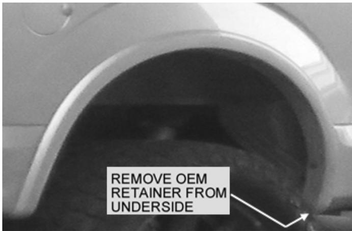
1. Remove the factory retainer from the bottom rear of the wheel well and discard.
