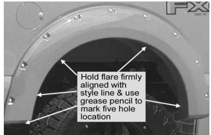
1. With a helper, firmly place the flare on the fender in the proper position and use a grease pencil mark the 5 hole locations in the fender well.
