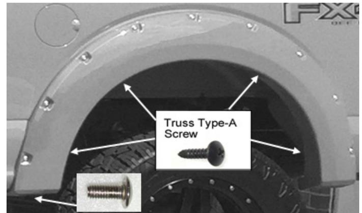
1. Again, mount the flare in the proper position on the fender and secure with 4 Truss Type-A screws through the long clips, starting with the 2 uppermost and working outward.
