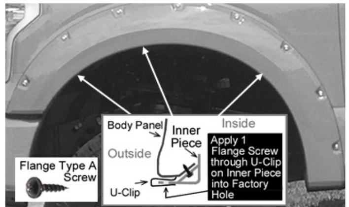
1. With a helper, firmly hold the flare in place on the fender, aligning the 3 uppermost mounting holes with the U-Clips on the inner bracket.
