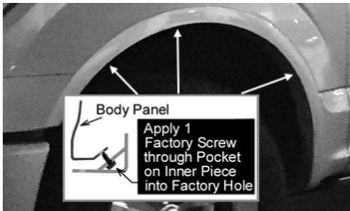
1. Be sure you have the correct inner bracket for the driver side and familiarize yourself with the proper location to mount. Line up the mounting holes in the inner bracket with the 3 uppermost factory holes.
