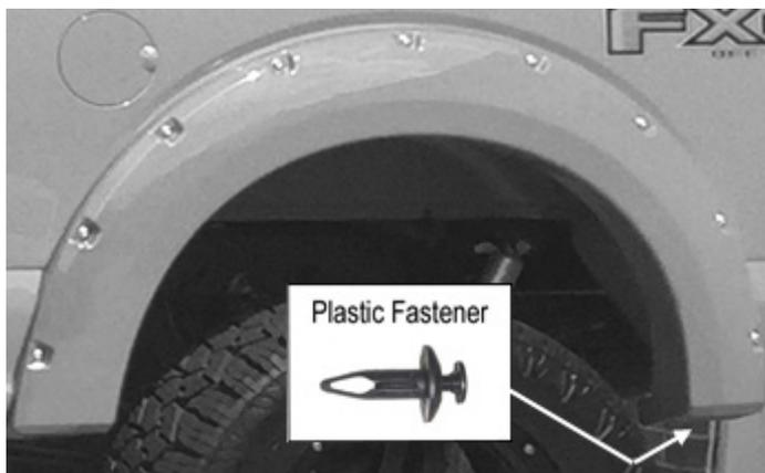
1. Apply one Plastic Fastener through the bottom rear hole of the flare and into the original factory hole.
