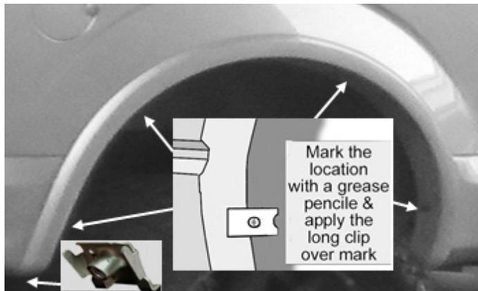
1. Remove the flare and apply four long clips over the marks made in the previous step
