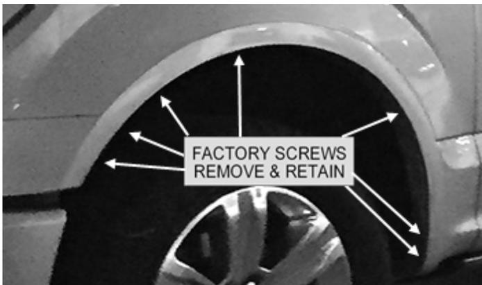
1. Remove the 7 existing factory screws and save for re-installation as shown.
