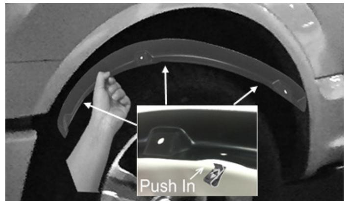
1. Install 3 U-Clips over the holes on the inner bracket as shown.
